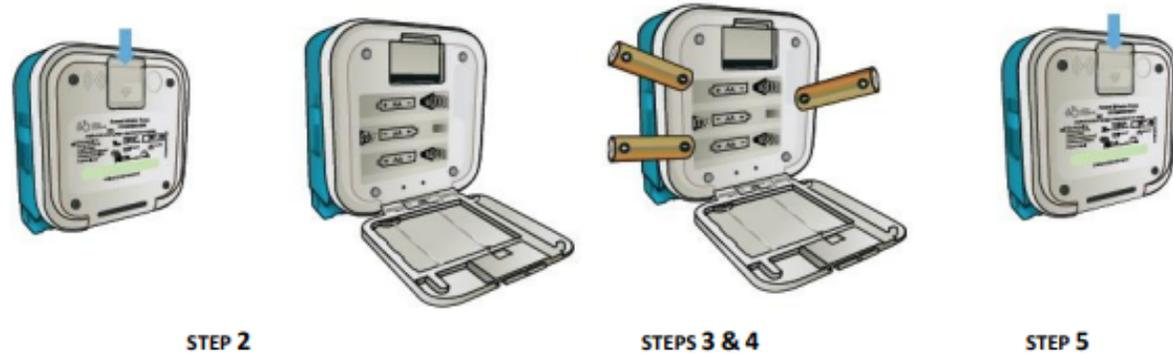
2. Open the battery compartment located at the pump's rear by sliding the latch downwards.
